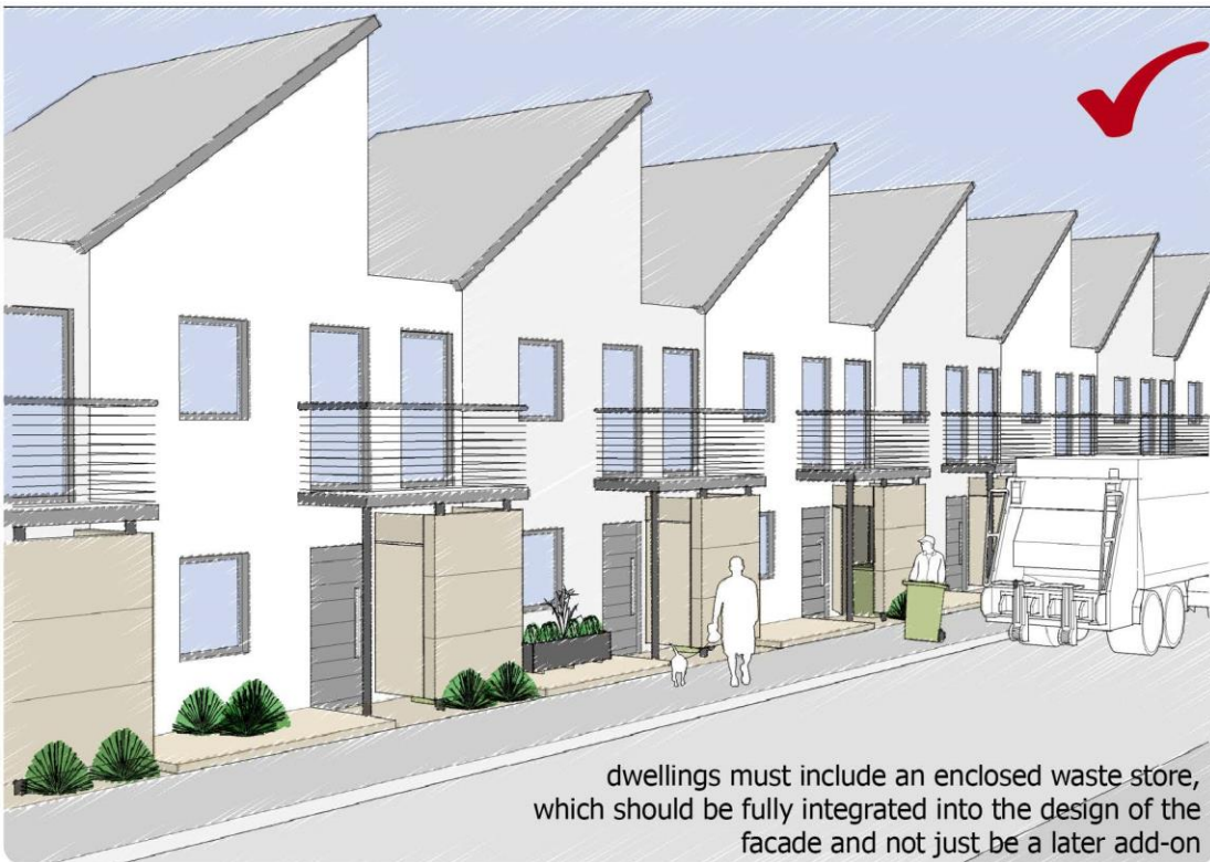
Figure 46: Good and poor examples of provision for bin storage in residential design
